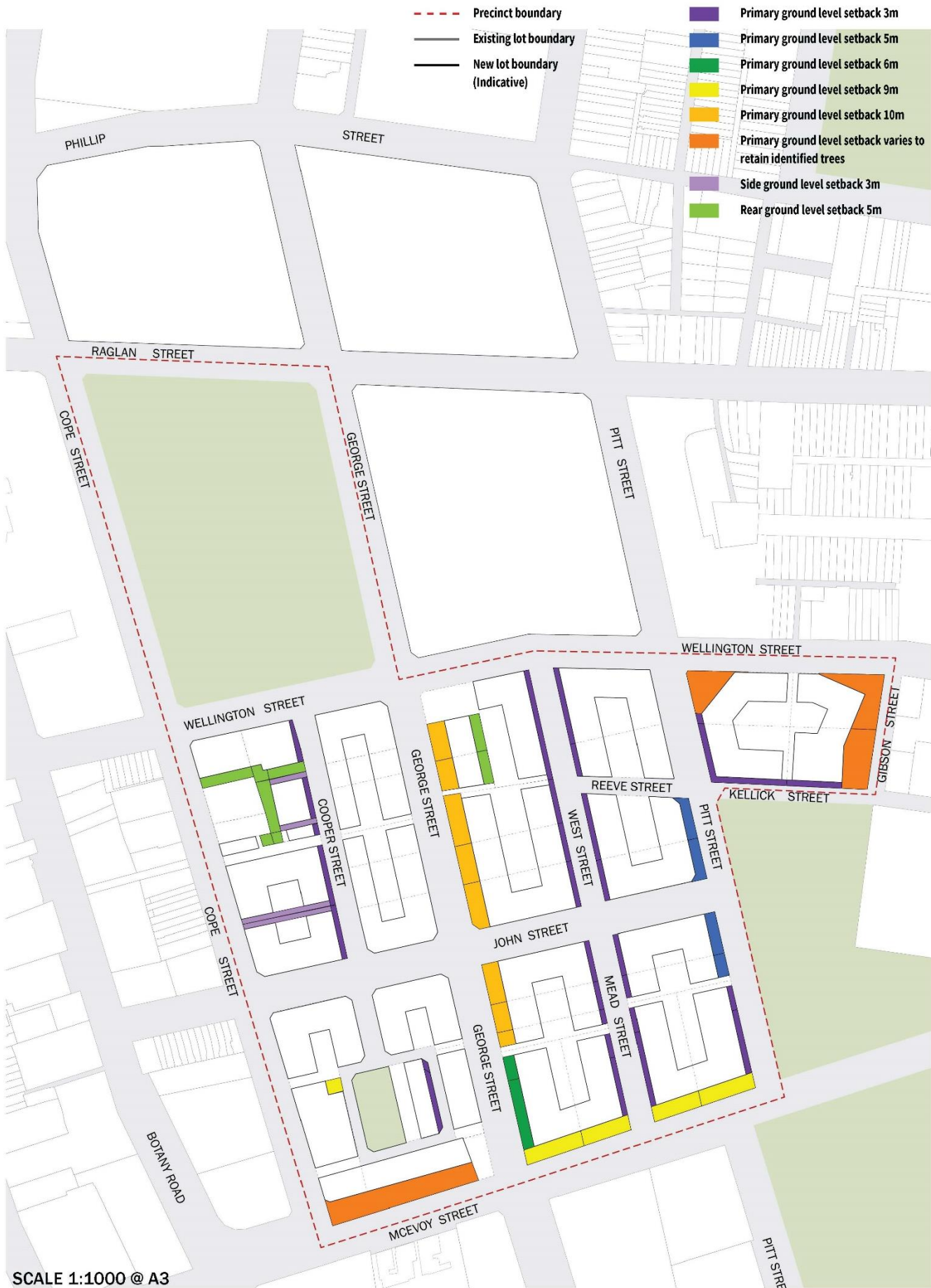
Figure 13: Ground level setbacks
